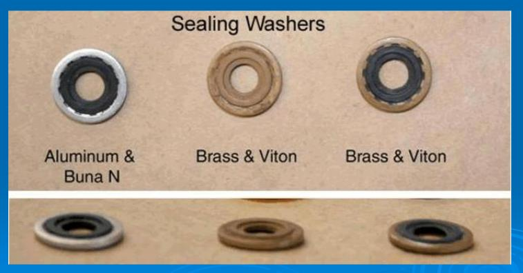
**Buna N:** Standard Nitrile is also known as Buna-N. Excellent resistance to petroleum-based oils and fuels, water and alcohols. Nitrile also has good resistance to acids and bases, except those with a strong oxidizing effect.
